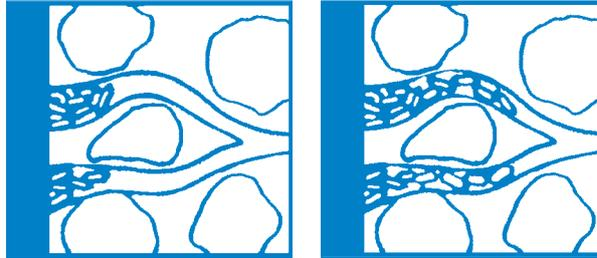
Crystals grow in the capillaries of cement based surface in damp conditions by 1cm/week up to a depth of 0.4 metres.
