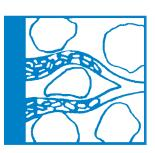
Crystals grow in the capillaries of cement based surface in damp conditions by Icm/week up to a depth of 0.4 metres.
