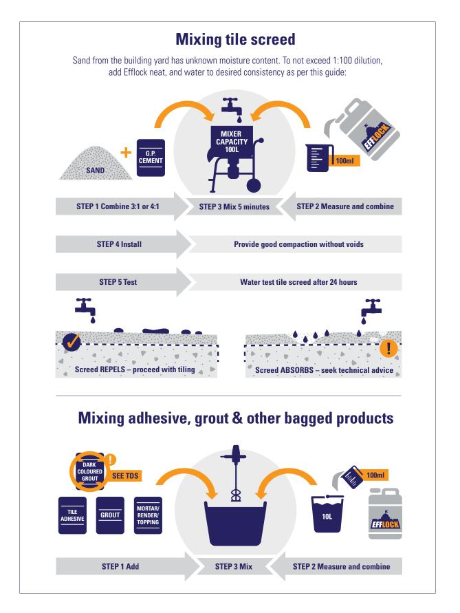
Efflock is a high performance, water based, VOC free, liquid additive designed for the bulk impregnation of cement based building materials to protect against efflorescence and damp.
